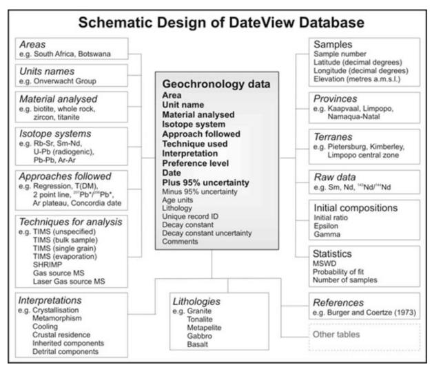
A main database table contains the principle information, but is supported by other, linked tables (bold, normal font in the diagram above). Numerous 'lookup' tables ensure referential integrity (bold, italic font in the diagram above).
